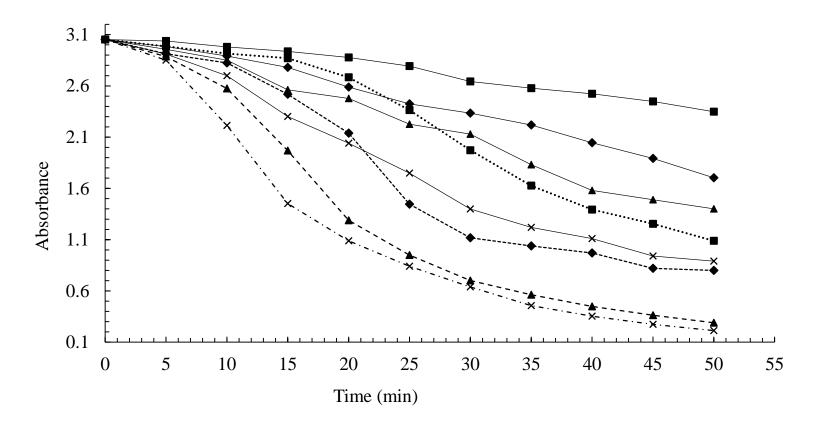
Absorbance change of diethyl (3H-1-ethoxy-3-phenoxazinylidene) ammonium chloride aqueous solution after exposure to an air plasma at atmospheric pressure (T) and at low pressure (T') as a function of exposure time and the electric current generating the plasma
