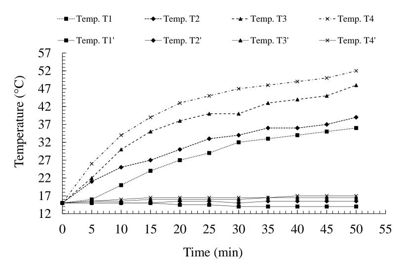
Change in temperature of the aqueous solution of diethyl (3H-1-ethoxy-3-phenoxazinylidene) ammonium chloride after exposure to an air plasma at atmospheric pressure (T) and at low pressure (T') as a function of the exposure time and the electric current generating the plasma
