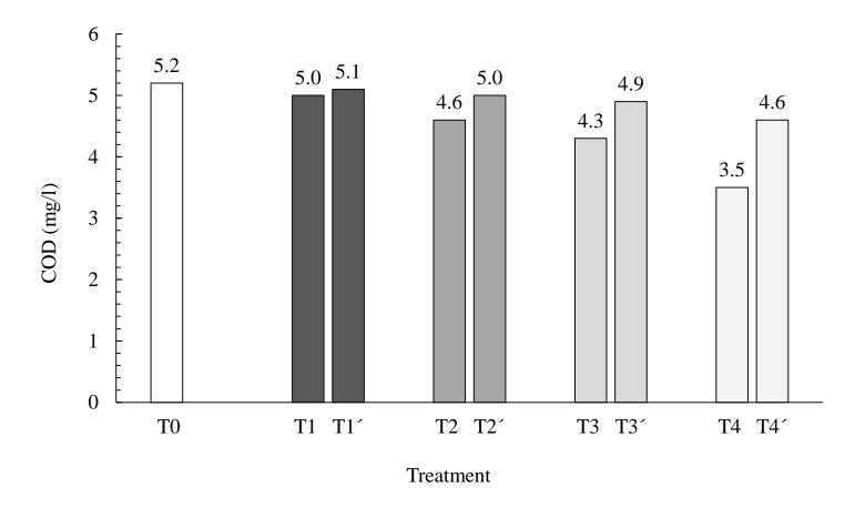
COD change of the diethyl (3H-1-ethoxy-3-phenoxazinylidene) ammonium chloride dye solution after exposure to air plasma as a function of plasma generation electrical power. To is the initial value of the solution of interest without treatment
