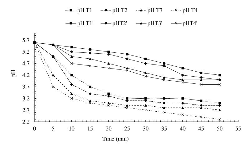
The behaviour of the pH change of the diethyl (3H-1-ethoxy-3-phenoxazinylidene) ammonium chloride dye solution, as a function of the exposure time to non-thermal plasma, the value of the electric current and the pressure in the reaction chamber. Atmospheric pressure (T) and low pressure (T')
